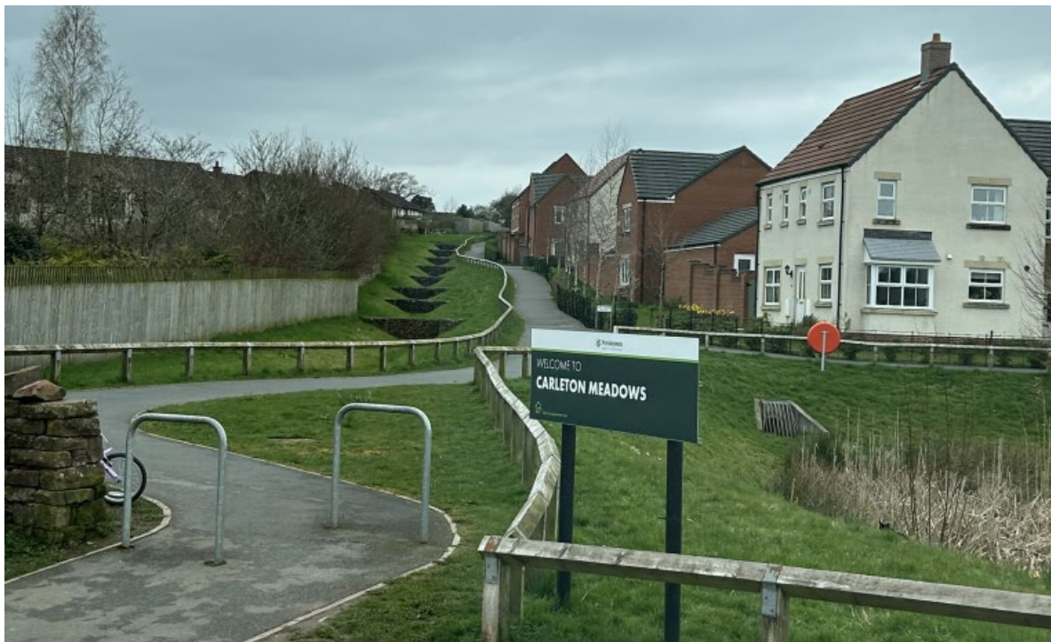
The stepped drainage channel in the centre of the photo becomes a water feature that slows down the flow of runoff in wet weather. It drains into the retention pond in the bottom right-hand corner. Penrith.
