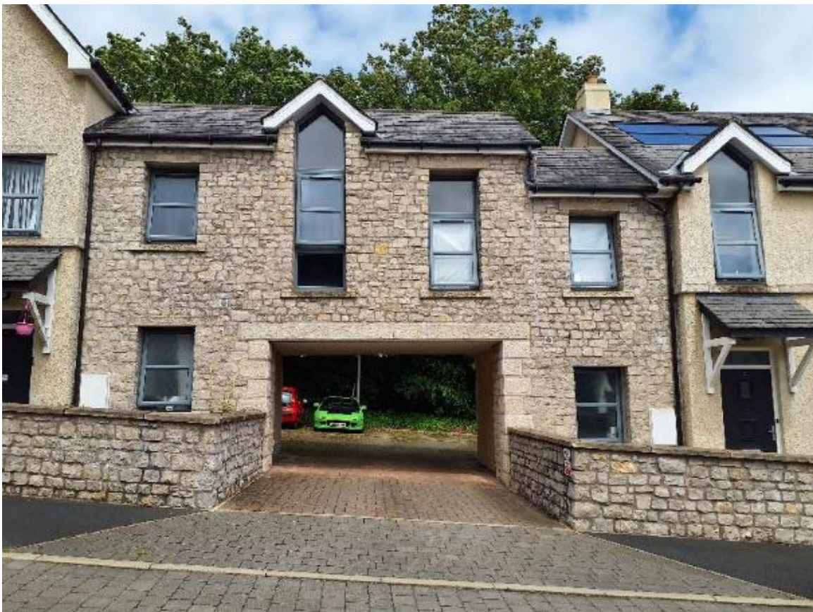
In the same development as the photo above, a concealed courtyard is another means of keeping the street free of parked cars. This in turn enables the street to be more traditional in its width and proportions. Grange-over-Sands.
