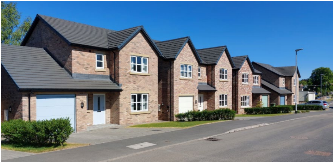
These homes at Langwathby are all lined up to form a building line, but with each house having different features set forward and recessed backward and having different designs, the building line is less pronounced.
