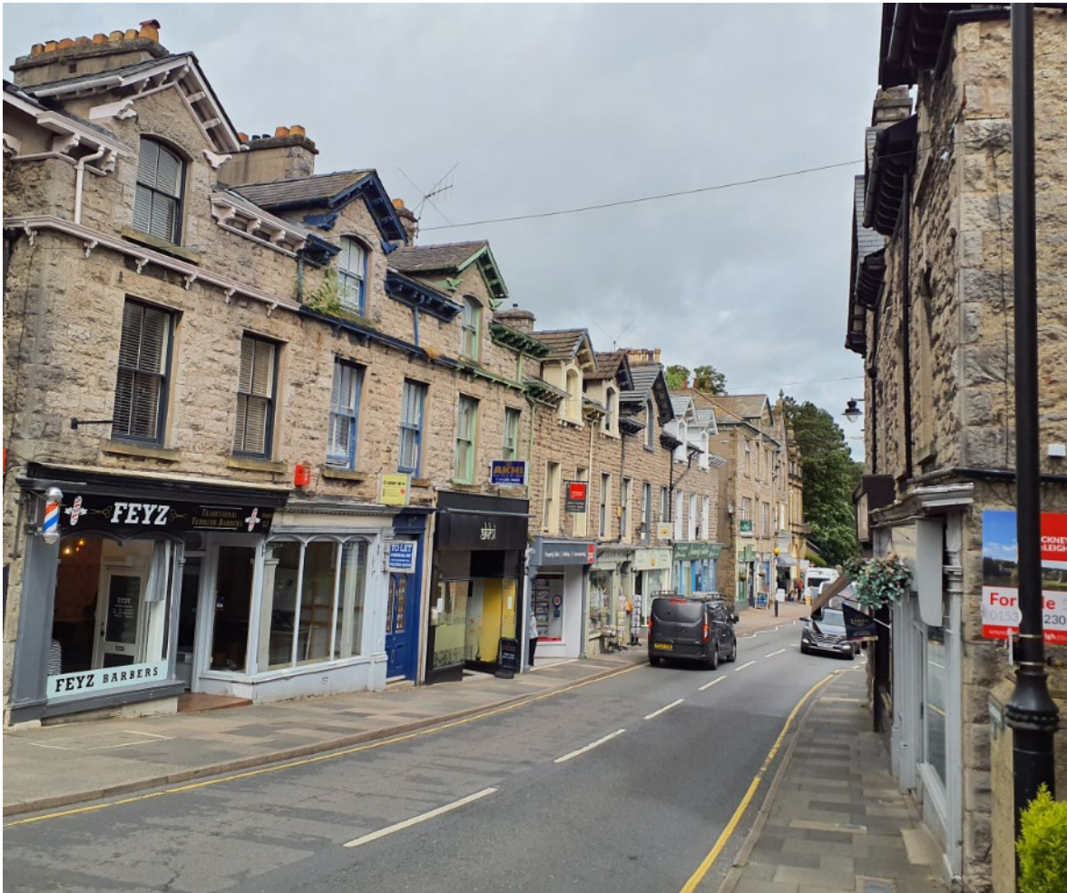
This primary street in Grange-over-Sands is a key through route, but is compact in its width, which helps to slow vehicle traffic down. The taller buildings and higher density emphasise the importance of this street.
