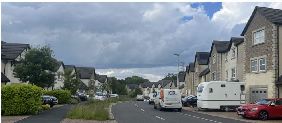
A planted verge offers amenity to the street, as well as providing a destination for runoff from the hard surfaces. Burton-in-Kendal.
