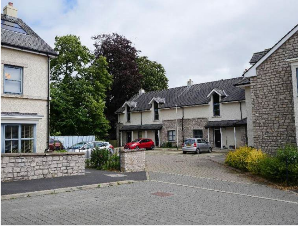
This small courtyard of parking is picked out in a different surfacing material. It keeps the adjacent street free of parked cars and pavement parking. Grange-over-Sands.
