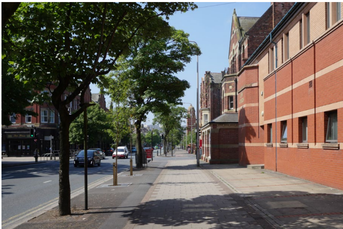
Here the strip of pavement space for the treeline is shared with signage, traffic signals and street furniture, leaving a clear, unobstructed and shaded space for walkers and wheelers. Barrow.
