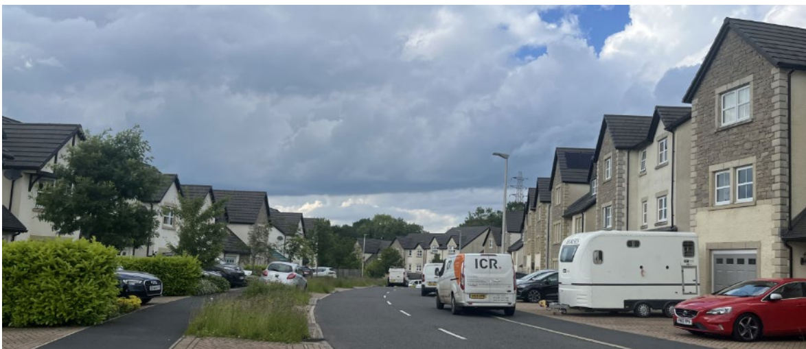
A planted verge offers amenity to the street, as well as providing a destination for runoff from the hard surfaces. Burton-on-Kendal.
